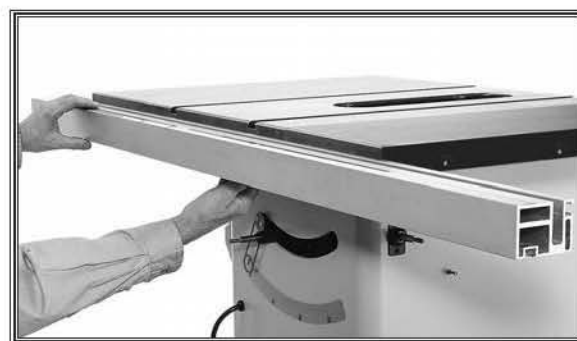
Figure 24. Mounting front fence rail.
