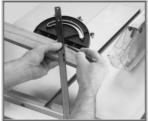
Figure 58. Example of marking miter line.
