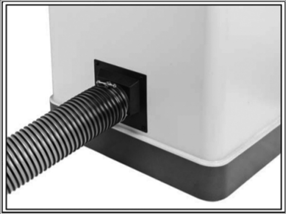
Figure 35. Dust port connected to dust collection system.
