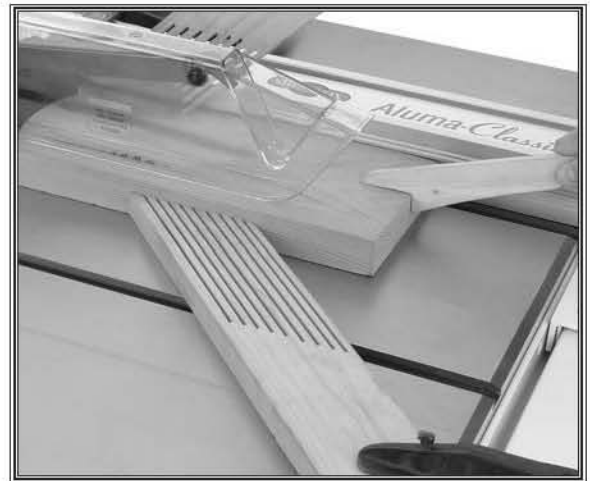
Figure 56. Typical ripping operation.
