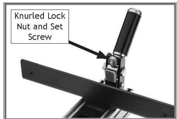
Figure 117. Set screw for adjusting fence handle clamping pressure.
