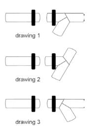
**The meaning of SUPRA** This word identifies the different type of clamps mounted on this welding machine. They have been specifically designed to be able to lock "branch" fittings: with extractable and interchangeable jaws, shaped according to the diameter to weld, it is possible to lock all branch points (drawings 1, 2, 3).
